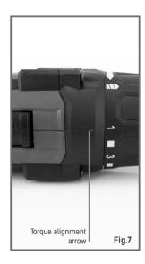
The torque setting required to drive screws will differ with different materials. Start with the torque setting on the number you think is appropriate (Eg: 4) and simply increase the torque adjustment collar to a higher number if the screw head is not sitting flush with your work piece. Remove the screw after adjusting and re-drive the screw back into the work piece until the correct torque adjustment leaves the screw head flush with your work piece.
